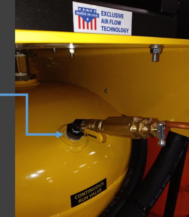
• INSTALL ¾" TO ¼" BUSING WITH THREAD TAPE OR SEALANT.
